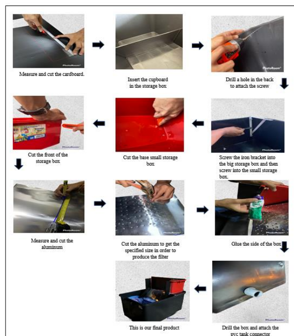
Figure 1: Flowchart Production of Smart Rubbish Bin with filter Box
